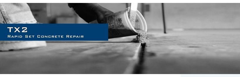
TX2 is a rapid set, high strength low viscosity urethane repair material. This two part, 1:1 system is 100% solids and designed for rebuilding and repairing broken control joints, filling voids under tile and concrete, and repairing spalled concrete surfaces very quickly. TX2 is intended for use in damaged control joints or warehouse spall damage created by forklifts or carts with steel or hard urethane wheels.
